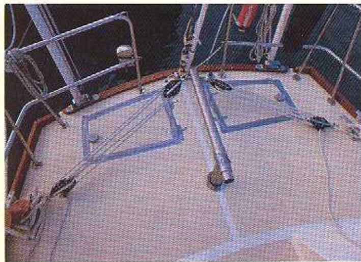
The emergency tiller shipped and the steering tackles rigged (left). Below is some idea of how we 'repaired' the original steering gear. The restraining tackle (bottom left) helps reinforce the arrangement at bottom right.
